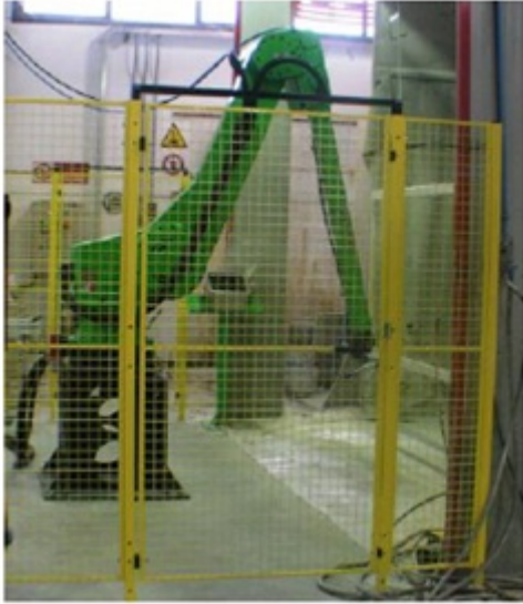
Figure 76:Perimeter fence 防护围栏
