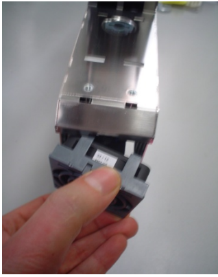
Figure94 Replacing the drives' cooling fans
